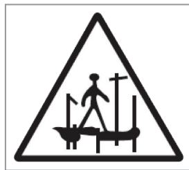
Danger Scaffolding Incomplete
